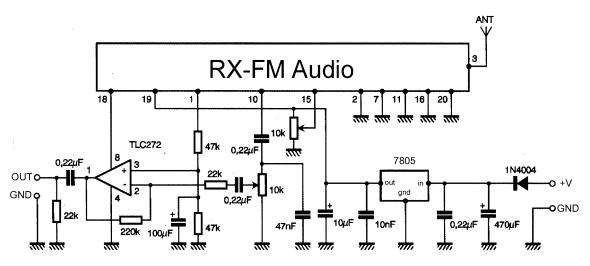
The above schematic diagram together with the TX-FM AUDIO transmitter module (see TX-FM AUDIO application notes) provides an example of a simplex voice communication channel where the receiver output can be fed directly into an external audio power amplifier.
