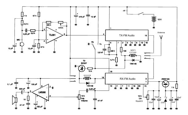
The schematic diagram above provides an application example using the RX-FM AUDIO receiver module together with the companion TX-FM AUDIO and interfacing components to make up a half duplex two-way radio or 'walkie talkie'.
