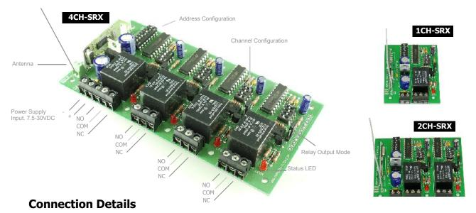
Power supply connection and relay outputs are all via the screw terminal blocks. The designation of each terminal is marked on the underside of the printed circuit board. The external power supply may be 7.5 VDC - 30 VDC, and be must be capable of supplying at least 500mA if all relays are to be energized simultaneously.
