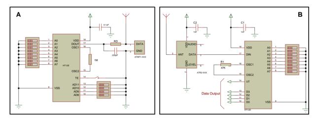
ATMT1 interfaced to HT12E data encoder (A) and companion receiver and data decoder (B)
