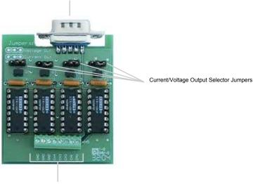
Supply Voltage, Ground and Outputs (Screw Terminals)
